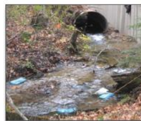
Figure 25. Six of the polymer blocks placed downstream
